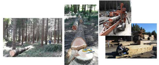
Standing trees are evaluated with portable ultrasound equipment and subsequently cut and processed. The timber boards and beams are again characterized with ultrasound and then sent to the laboratory to obtain the reference values
